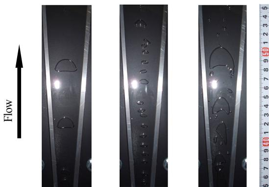
Fig. 7 Flow configurations in the diverging channel<sup>19)</sup>.
