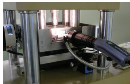
Photo 4 Observational system of shear band with CCD microscope
