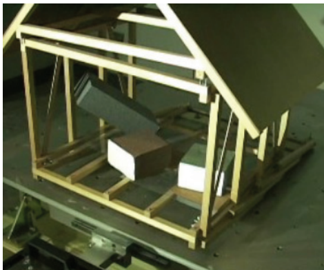
Photo 5 Animation of wooden house model without bracing in the first story
