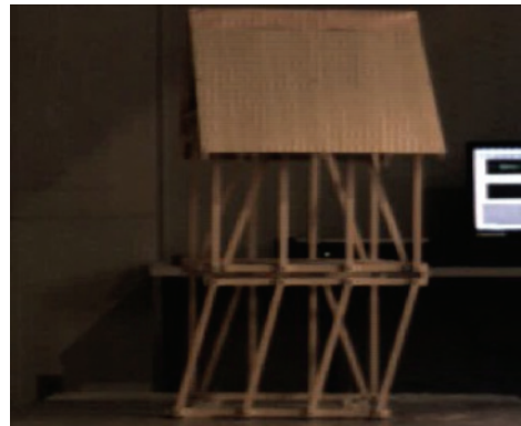
Photo 3 Animation of wooden house model with bracing only in one side
