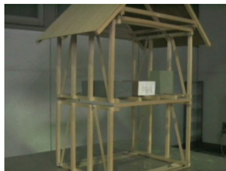
Photo 9 Animation of fall of furniture in wooden house model with bracing in both sides
