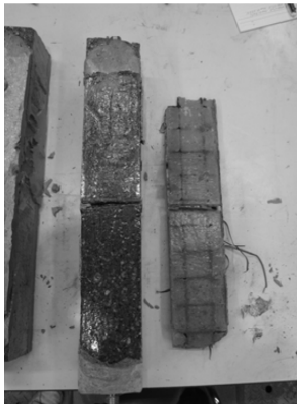
Photo.2 The specimen with CFRP grid (1 Layer).
