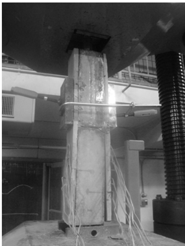
Photo.1 The specimen after FRP debonding.
