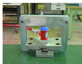
(a) Removing the upper shear box
