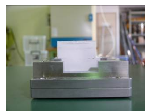
(b) Taking out of the upper shear box
