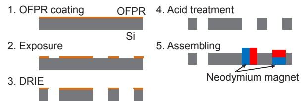
Fig.3 Fabrication process of on-chip robot.
