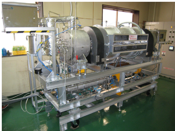
Fig. 15 Rotary kiln apparatus for mass producing MWNTs.
