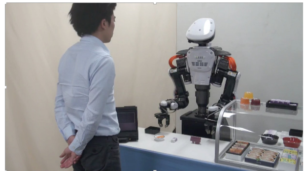
Fig. 4 Example of service robot system based on RTCs with HIRO
