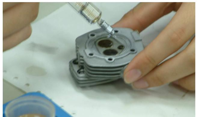
Fig.5 Measurement of Combustion Chamber Volume
