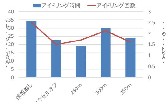
Fig.17 Idling times and number of idling
