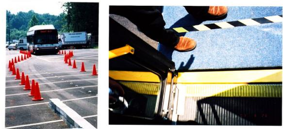
Fig. 2 An automated bus by California PATH: (left) the bus drives along the narrow path defined by road cones. A series of objects at the middle of the path are magnets for the lateral control; (right) the bus performs precision docking.
