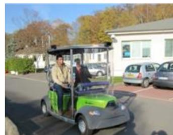
Fig. 5 A low-speed, small autonomous vehicle for the transportation poor developed by INRIA.
