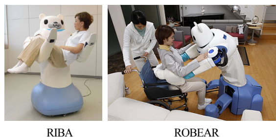
Fig. 1 Nursing-care assistant robots we developed.
