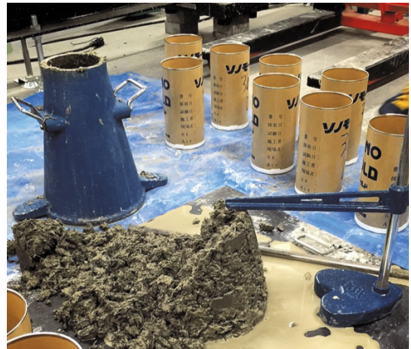
Fig.5 Slump test result (24N-F0%)
