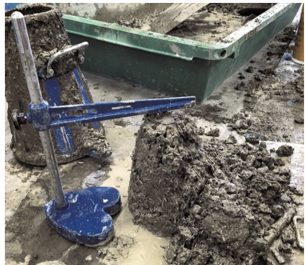
Fig.7 Slump test result (30N-F0.5%)
