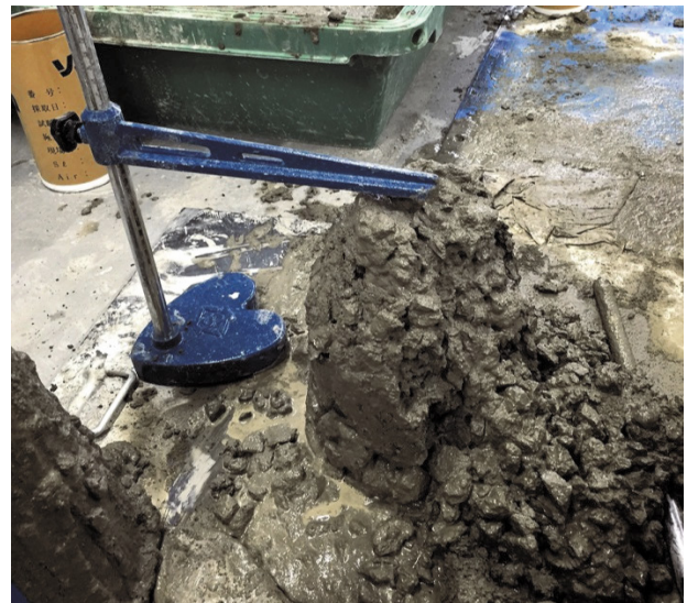
Fig.6 Slump test result (40N-F0%)
