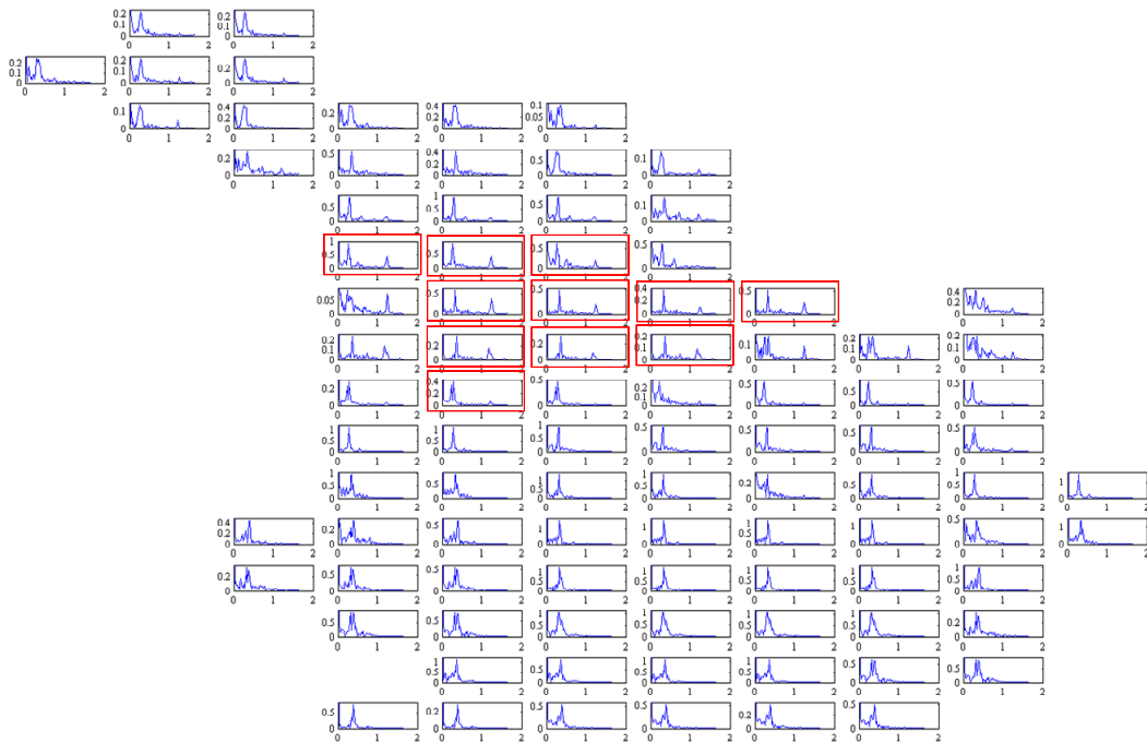
Fig. 6 Spectra of pressure time series from different cells when a human in prone posture is on the sensor. Cells without pressure are omitted.
