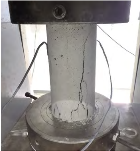
Photo 4 Test set-up of compression test N specimen.
